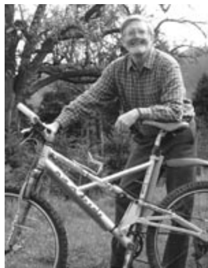
Colin Palmer with his full-suspension Marin: disk brakes, 27 gears, light weight, and a suspension system that increases rideability and decreases punishment to ageing wheelmen.
